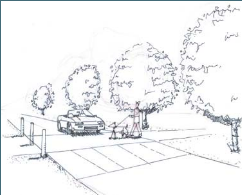
Raised Pedestrian crossing
