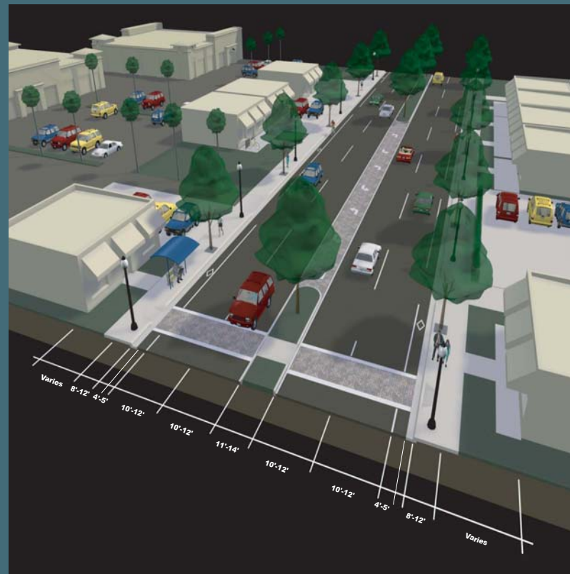
Continuous left turn line/bicycle lane
